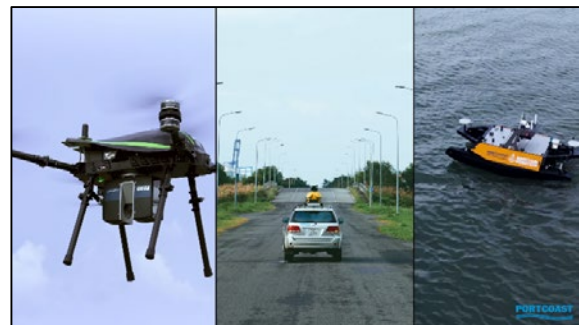
Figure 6 Mobile mapping systems mounted on vehicles and unmanned aerial vehicles technology combined with sensors like LiDAR, Laser Scan and Unmanned Surface Vehicles combined with Multibeam echo sounding or LiDAR
