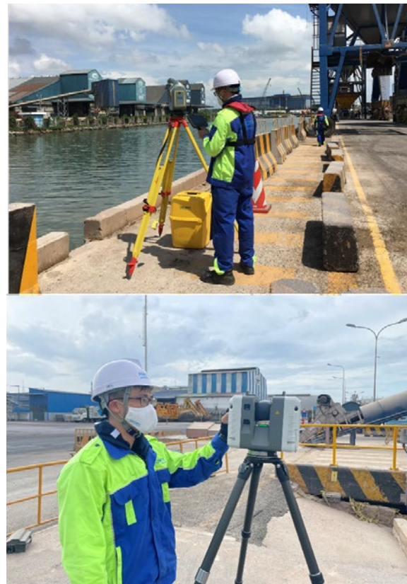
Figure 2. Multi-station SX12 on the wharf (top) and Leica RTC360 under the pier (bottom) for laser scanning
