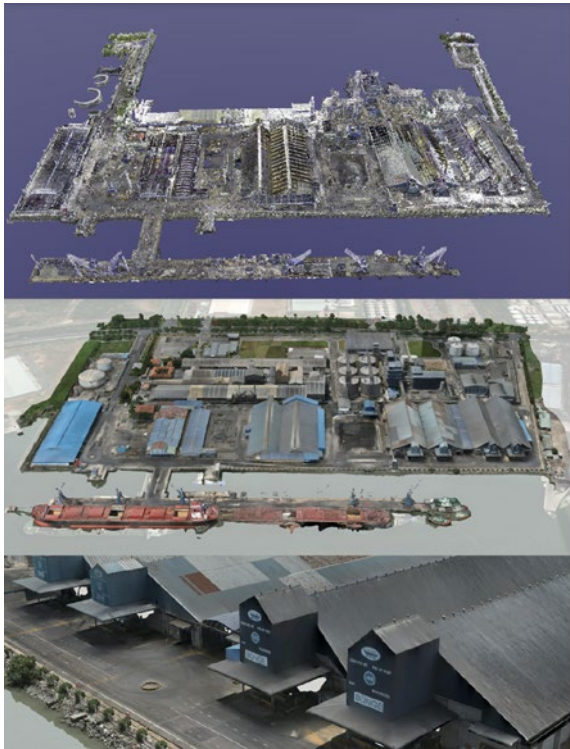
Figure 8. 3D point cloud model (top), 3D photogrammetry model (middle) of Baria Serece port, and zoom in a part of 3D photogrammetry model (bottom)
